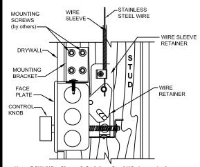
Note: BCW (Wire Sleeve & Stainless Steel Wire) must be in as straight line as possible from damper to insure optimum performance. Wire and casing between damper and controller should be secured every 4 feet.
